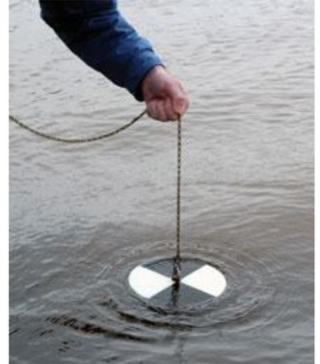
Scientists and citizens can measure turbidity by lowering a device called a Sechi (pronounced seh-key) Disc into the water. It is a round metal disc, painted black and white. Turbidity is determined from the depth in which the disc is lowered and "disappears" from view. In estuaries, the Sechi Disc may only be lowered four or five feet before it disappears from view. In the Gulf Stream with few particulates, the Sechi Disc may be lowered 100 ft.
